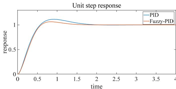
**Fig 4.** Comparison curve of PID algorithm and fuzzy PID algorithm in the horizontal direction
