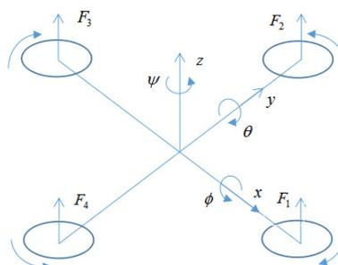
**Fig 1.** Schematic diagram of quadrotor UAV model
