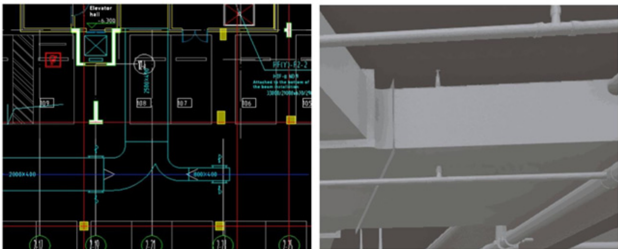
Figure 3. Air duct and spray pipe collide, and the intersection of axis D of axis C and axis C of B
